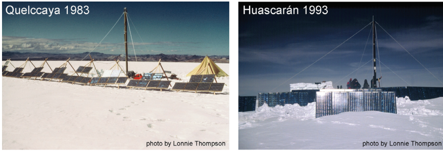
FIGURE 1. Lightweight, solar-powered drilling systems (Quelccaya 1983, left; Huascarán 1993, right), which made deep drilling on high-elevation tropical glaciers possible.
