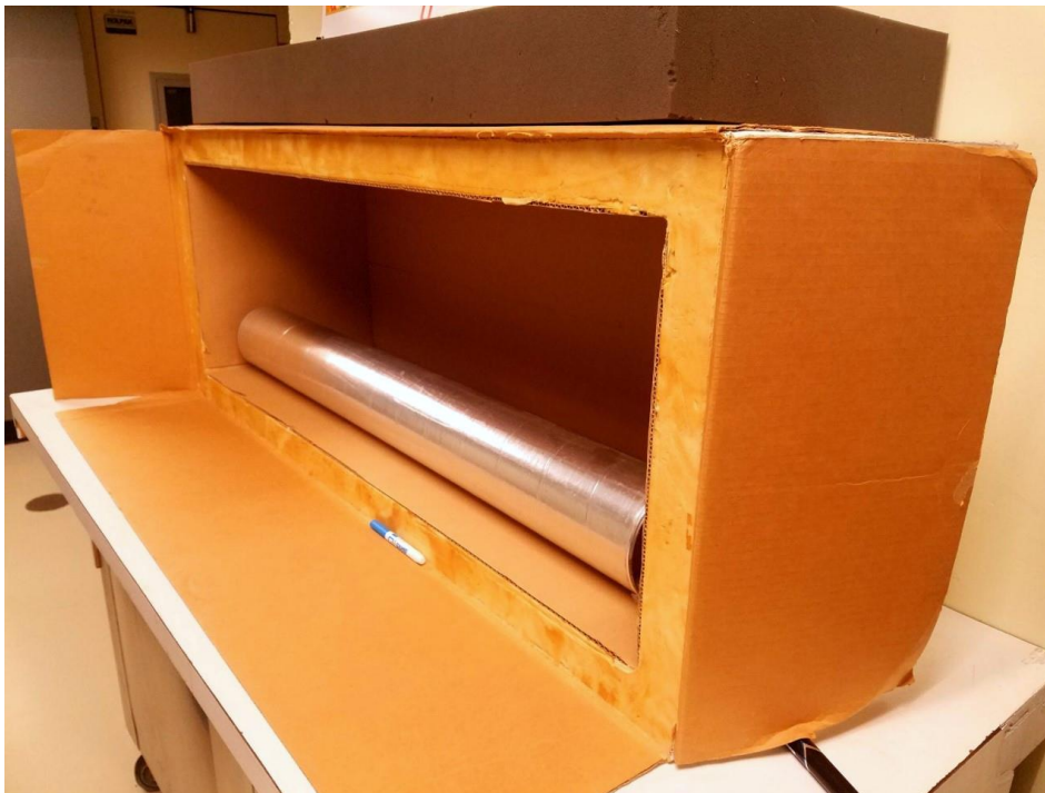
Cardboard box with Styrofoam and ice core tube to represent the general structure of an ice core container for transport and storage. Credit: Byrd Polar and Climate Research Center
